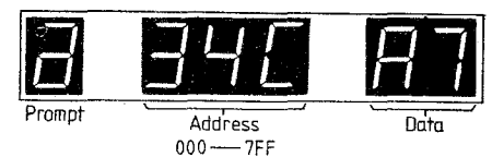
Fig. 1. A typical display. The 8060 processor has only 12 address lines, hence the hexadecimal address display consists of only three digits.
