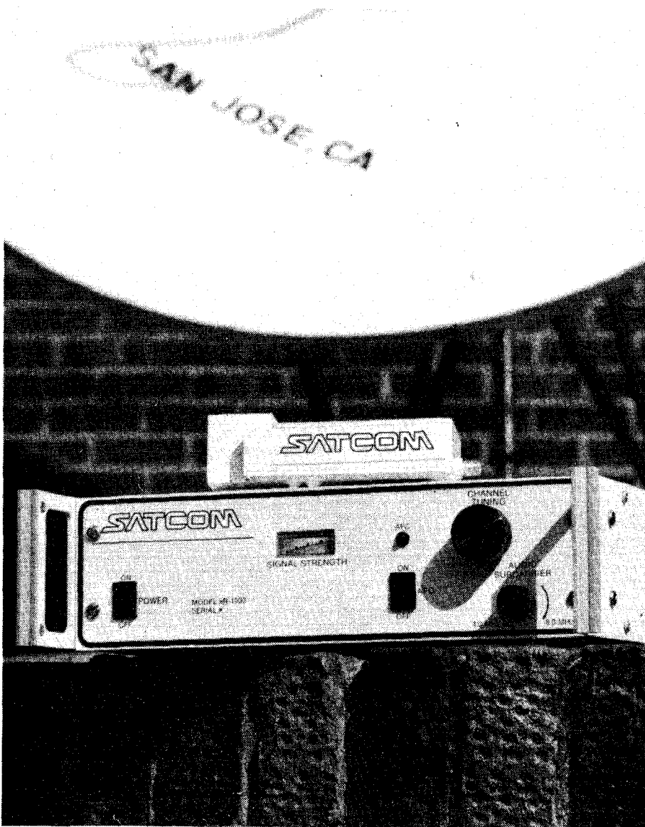
Satcom 1200 is a 12GHz receiver for direct broadcasts from satellites. Signals received from the dish aerial are amplified by a low noise downconverter using Gallium Arsenide fetts and hybrid i.cs. To give a stable low-drift performance across a minimum 500mHz bandwidth. The signals are fed to an indoor tuner with a further downconversion to normal broadcast frequencies, which are demodulated to PAL - G/625 line standard. For use on future DBS the dish size may be as small as 700mm but for current satellite transmissions, dishes of 2 to 3 metres are offered. The system is marketed by March Microwave in Braintree, Essex.
